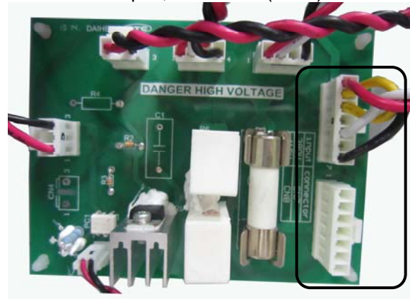
CN8 open, CN7 wired (380V)
